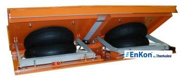
Dual tilt modules are used for extra long racks. Capacities up to 14,000lbs can be achieved. Continuous piano style hinge provides stability and safety by eliminating pinch points.
