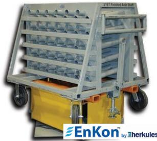
Enkon Cart Lifts allow your push carts to be positioned at the correct ergonomic heights. With each cart lift designed and built to your exact cart specifications, flawless integration is guaranteed.
