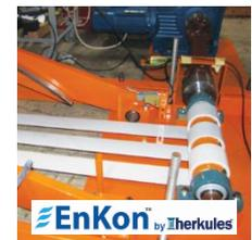
**Safety bellows skirting** – To protect from pinch points and debris.
