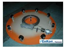
Spiral Gear Drive The gear drive utilizes precision accuracy with automatic locking when not under power.
