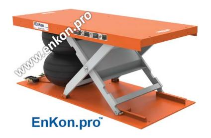
Featuring a narrow width and long platform at  $31" \times 71"$ , the LSA29 Air Scissor Lift Table provides a raised height of 29", and 25" travel. Positioning the air bag next to the scissors allows not only a profile under 5", but also a lift capacity up to 5000 lbs.
