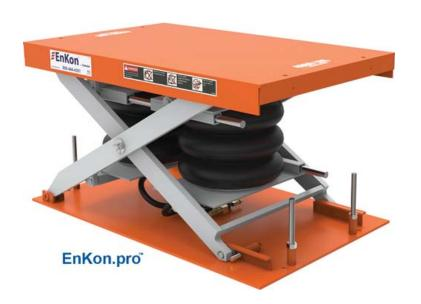
Improving ergonomics within a narrow footprint, the LSA24 Air Scissor Lift Table offers a 29" x 47" platform and a lift capacity up to 4000 lbs. This lift, with two triple air bags, provides a 25" raised height, under 10" profile, and 16" of travel.
