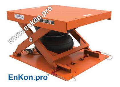
Part of the Herkules super duty family, the LSA21 Air Scissor Lift Table is a heavy-duty pneumatic scissor lift table with a raised height of 32". Built with 3/4" thick top and bottom plates, featuring a 44"  $\times$  52" platform, a low profile of 7" and 25" travel, the LSA21 raises up to 10,000 lbs.
