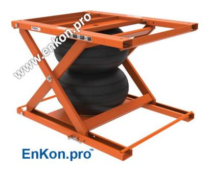
With double the lifting capability of the LSA14, the LSA17 Air Scissor Lift Table can lift up to 6000 lbs. and offers a lightweight construction with superior welds. The lift provides a 31" raised height, 7" profile and 24" of travel, with dimensions of  $36" \times 47"$ .
