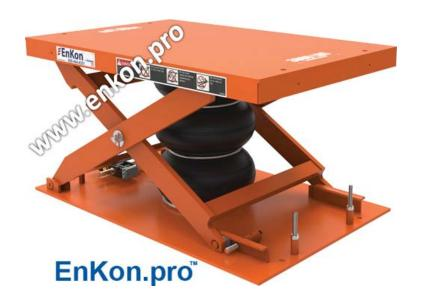
Fork-free environments get the lift they need with the LSA04 Air Scissor Lift Table. Ideal for positioning carts, this pneumatic lift has a 6" profile, 15" of travel, a raised height of up to 21", and platform dimensions of 25" × 40". Powered by a small airbag, the LSA04 provides a one-to-one lift ratio, with the capability to lift up to 3000 lbs.
