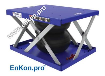
The original Enkon four-scissor, low-profile lift, the LSA01 Air Scissor Lift Table is powered by Herkules-patented air bag technology and employs a direct, one-to-one lifting ratio. This powerful lift reaches a raised height of 29", and has a lowered height of only 4". The LSA01 provides a lift capacity up to 6000 lbs., and a platform of 38" x 50", and has 25" of travel.
