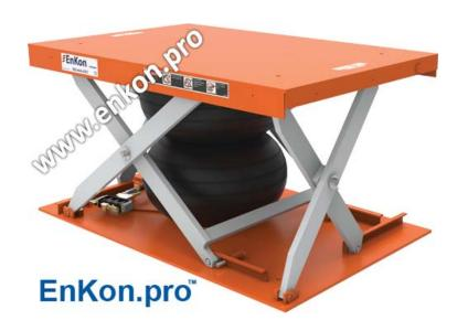
An incredibly stable 4 scissor pneumatic lift that excels in handling side loads, the LSA40 Air Scissor Lift Table is both compact and reliable. Similar to the LSA25, the LSA40 provides the same low profile of 4" and a smaller platform of 36" x 57". With up to 25" of travel, the LSA40 offers a final raised height of 29" and can lift up to 6,000 lbs.
