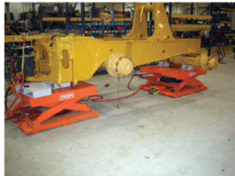
Two heavy duty, high capacity air lifts are synchronized to raise a back hoe easily and move it up/down the assembly line with air casters. (V0424)
