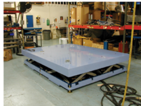
A high capacity lift system, built to lift and move rocket ships, is equipped with air casters allowing a 20,000 lb load to be pushed around the plant floor easily. (VP0002)
