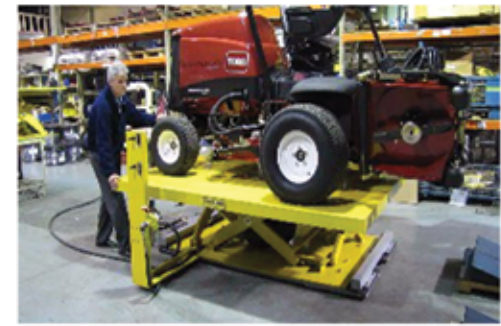
A portable, heavy duty scissor lift table, used for assembling Toro equipment, can be easily moved from station to station by use of air casters mounted to the base of the system. (V0752)
